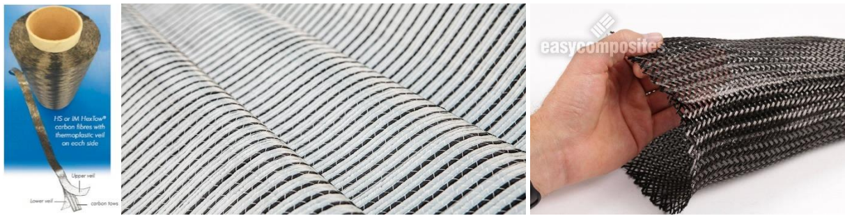
Figure 12: Examples of complex materials: Hexcel UD tape and Non-Crimp Fabric, and an Easy Composites braided sock
